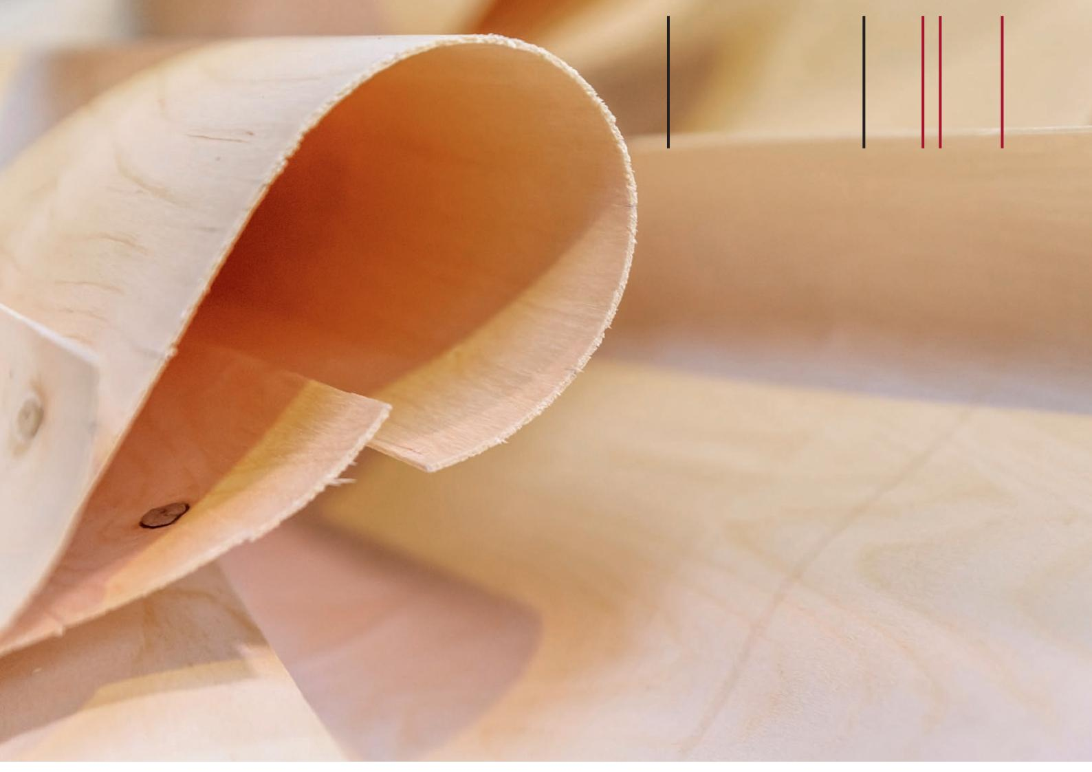
**Riga Combi is a plywood composed of birch and alder veneer layers, available as Riga Ply Combi, Riga Form Combi and Riga Tex Combi.**
